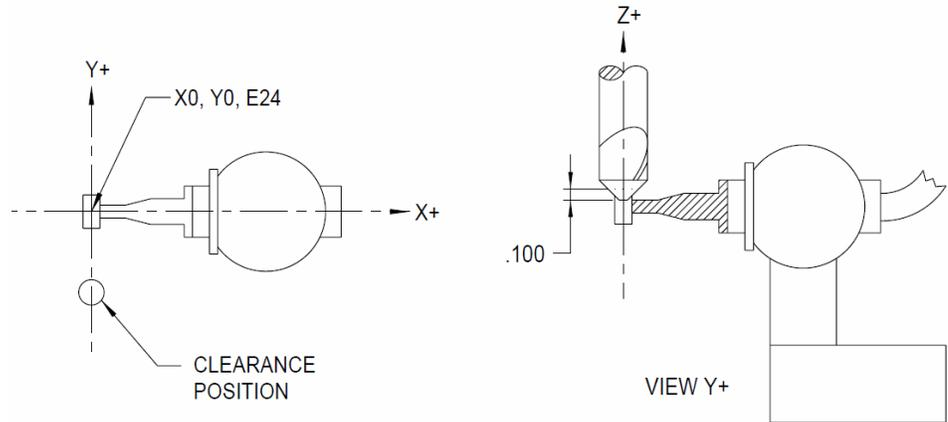
**Figure 15-11** Clearance Position & Touch Probe Selection
