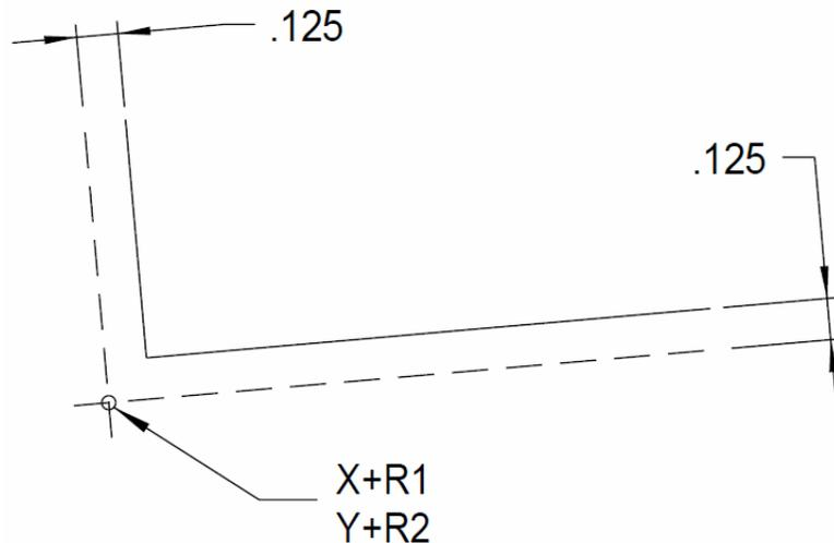
**Figure 15-19** CNC Movement to Corner
