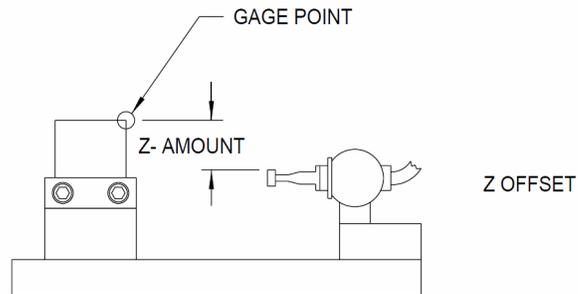
**Figure 15-7** Z Fixture Offsets
