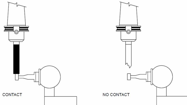
**Figure 15-24** Tool Breakage Detection
