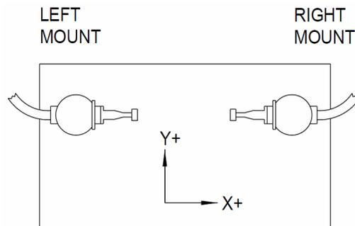
**Figure 15-5** Probe Mounting Positions
