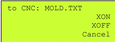
When the Software flow control method is used, the current XON or XOFF that has been received during transmission will be displayed on the right of the display. Use this feedback to determine if the USBCNC unit is receiving XON or XOFF characters.
