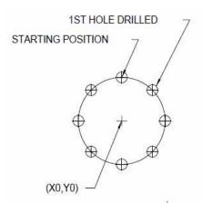
Figure 6-3 1st Hole Drilled
