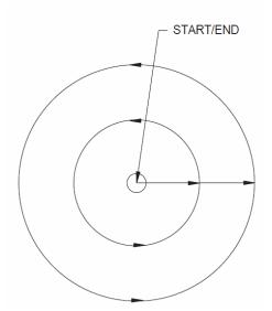
Figure 6-8 Counterclockwise Circular Pocket Clean-Out
