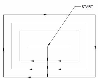
Figure 6-7 Clockwise Rectangular Pocket Clean-Out
