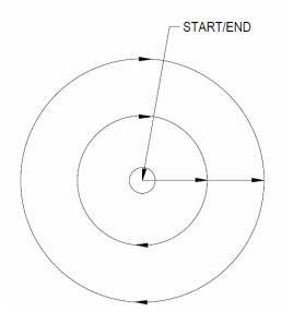
Figure 6-9 Clockwise Circular Pocket Clean-Out
