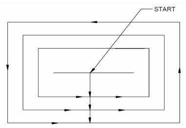
Figure 6-6 Counterclockwise Rectangular Pocket Clean-Out
