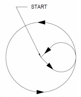
Figure 6-4 Boring Cycle Counter Clockwise
